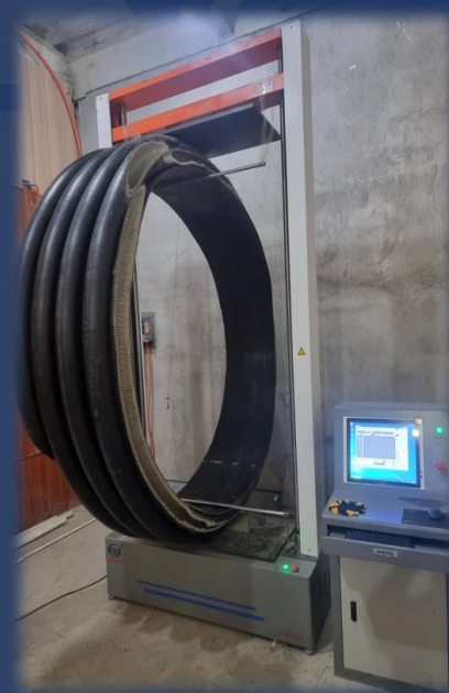
Tigershield Plant Conduct testing for the Ring Stiffness of the Carat Structured Wall HDPE Pipe.
